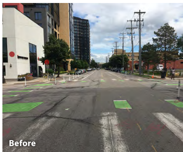
Figure 25: Paint and bollards improve conditions for people walking and bicycling; 11th Avenue and 2nd Street S
