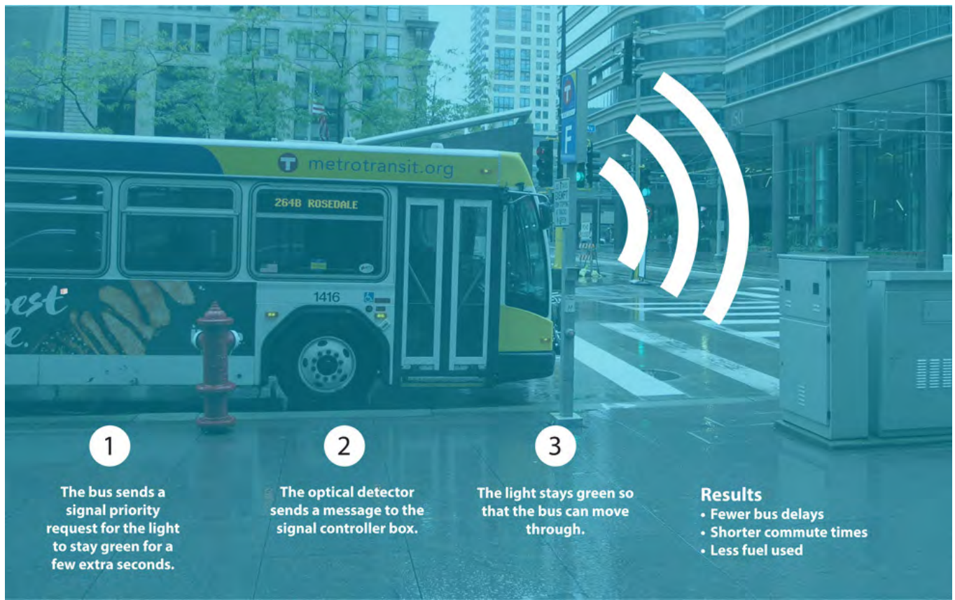
Figure 79: Transit signal priority
